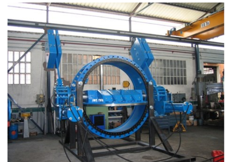
Overspeed valve DN2000 PN25, double arm
