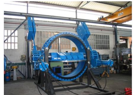
Overspeed valve DN2000 PN25, double arm
