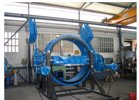
Overspeed valve DN2000 PN25, double arm
