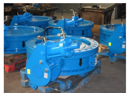
Check valves DN900 PN16 with hydraulic shock absorber
