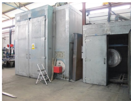
Polymerization ovens, 3x3x5 meters
