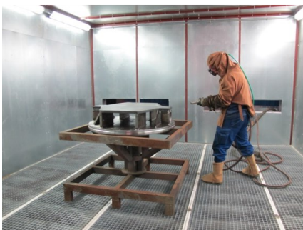
Manual blasting cabin 4.5x4.5 meters
