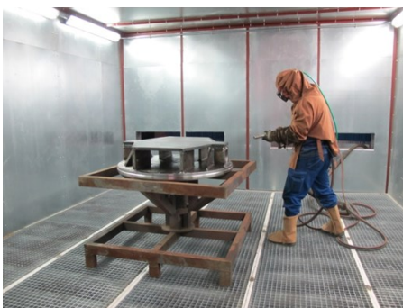
Manual blasting cabin 4.5x4.5 meters
