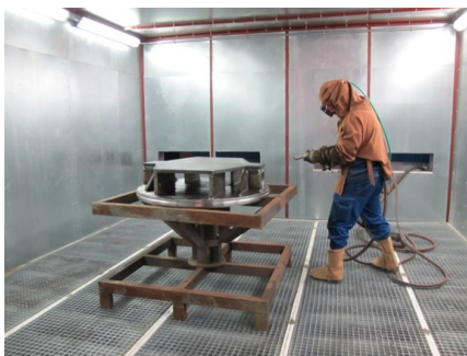
Manual blasting cabin 4.5x4.5 meters
