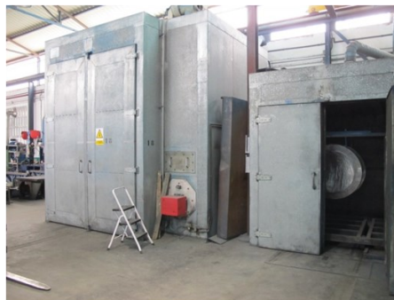
Polymerization ovens, 3x3x5 meters
