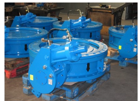
Check valves DN900 PN16 with hydraulic shock absorber
