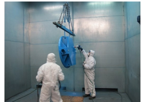
Manual powder coating, cabin 4x4 meters
