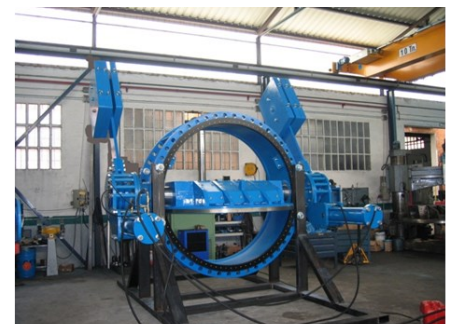
Overspeed valve DN2000 PN25, double arm
